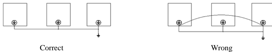
Figure 3-8 Grounding Wire Connection Sketch Map
